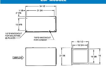
Electrical: 115/1/60, 0.25 amps Output: 12,000 VDC, 5.0 MA Max Weight: 88 lbs. Full; 53 lbs. Empty
