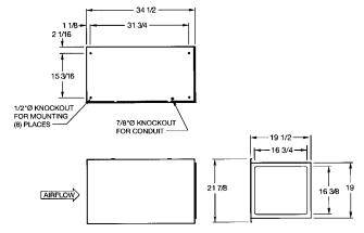
Electrical: 115/1/60, 2.0 amps Output: 48 UV watts with 1.4 amps
